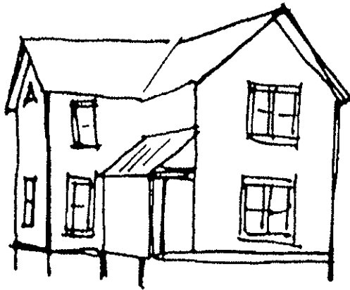
Roof pitches - 4:12 to 12:12, Shed roof - 2:12.
