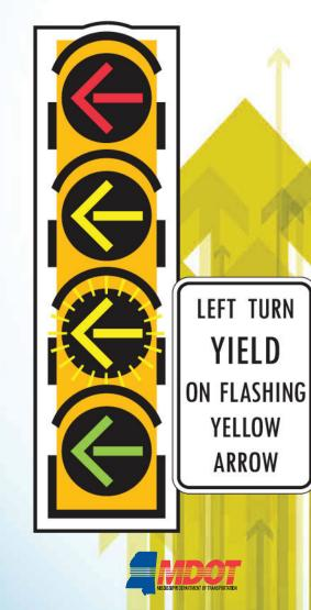
The Mississippi Department of Transportation (MDOT) is implementing a new traffic signal to provide a safer, more efficient left-turn for motorists. The Flashing Yellow Arrow left-turn signal is a new type of display that will begin to replace the circular green signal for permitted left-turns at selected intersections.
