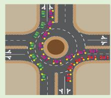
This graphic shows appropriate travel paths when using the correct lane in the roundabout based on these guidelines.
